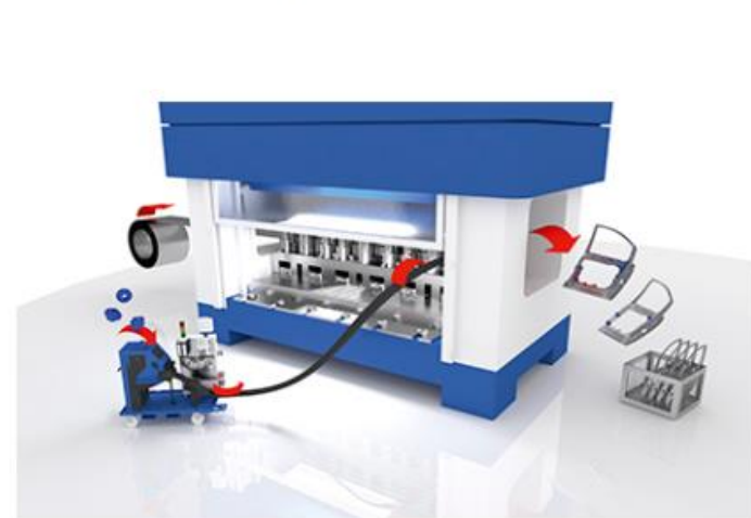
Fully automatic placement
